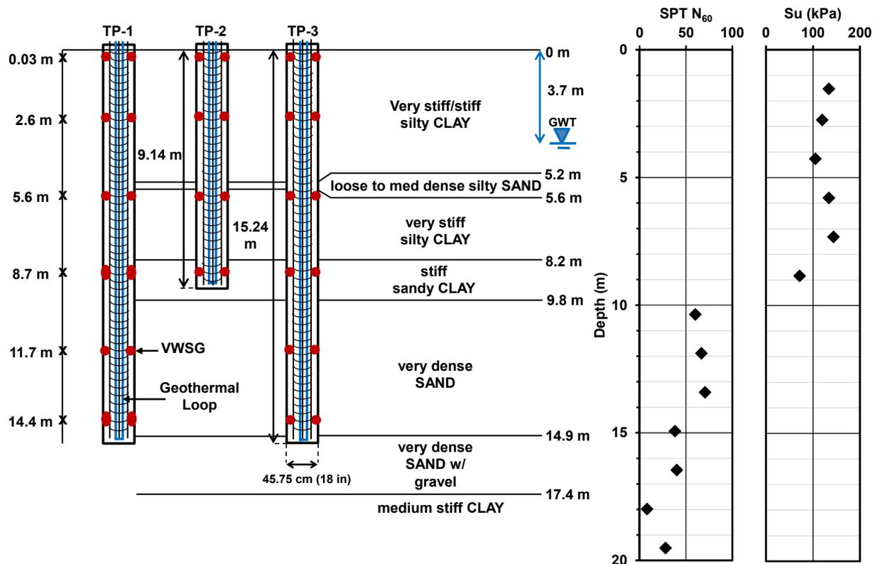
Figure 1. Test piles and soil profile.
