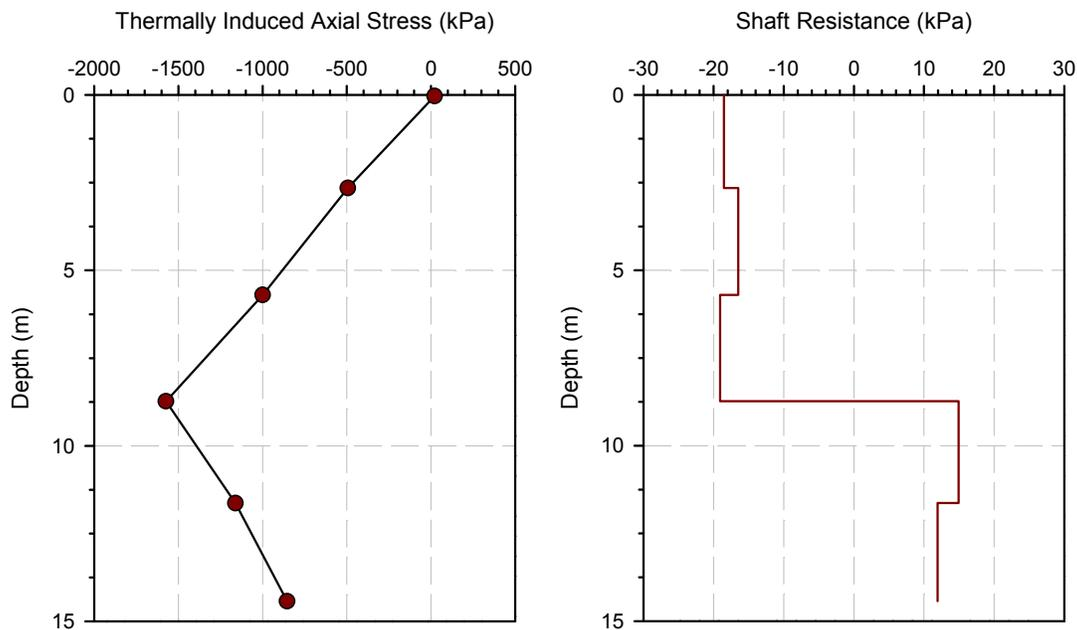
**Figure 6. a) Thermally induced axial stresses b) Mobilized shaft resistance along TP-1.**
