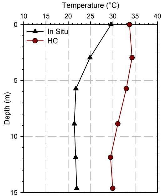
Figure 7. Temperature profiles along TP-3.
