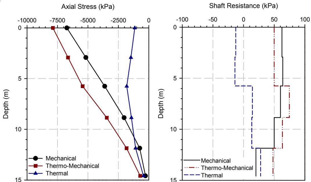
Figure 8. a) Thermally induced axial stresses b) Mobilized shaft resistance along TP-3.
