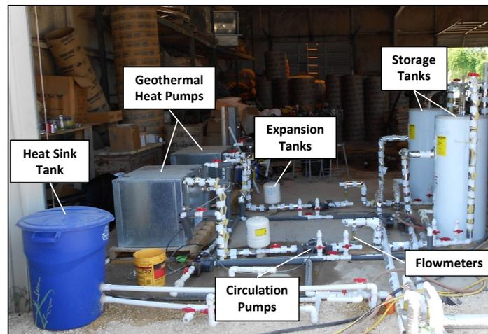
**Figure 2. Equipment used for thermal load applications.**
