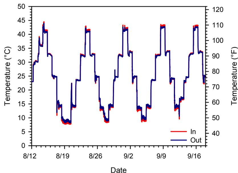
**Figure 3. Temperature cycles applied to TP-1.**
